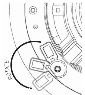
If your speaker includes a pivoting tweeter aiming it toward the listening area will raise the amplitude of the highest frequencies (>12kHz), adding brilliance. USE CARE TO AVOID DAMAGING THE DOME OF THE TWEETER WHEN AIMING!
